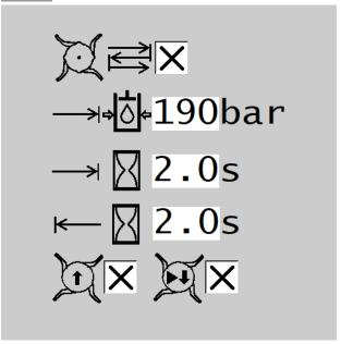
Auto-reversing can be enabled for the windrower and feed rotors, when activated the rotors will reverse for a adjustable time when a specific pressure is reached for a specific time. Autobalance must be active for Auto-reverse to activate.
