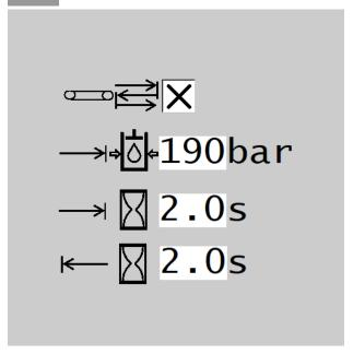
(Sideflow model only) Auto-reversing can be enabled for the elevators, when activated the elevators will reverse for an adjustable time when a specific pressure is reached for a specific time. Elevator Auto-reverse can be activated when the elevators are running in the forward direction. The elevators can be started by softkey, AUX-N Button or AUX-N proportional input.
