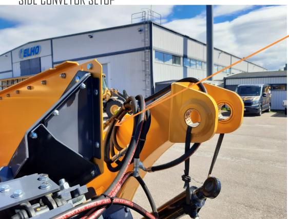
The hoses that attach to the two cylinders lifting and lowering the side conveyor is located at rear right hand side.
