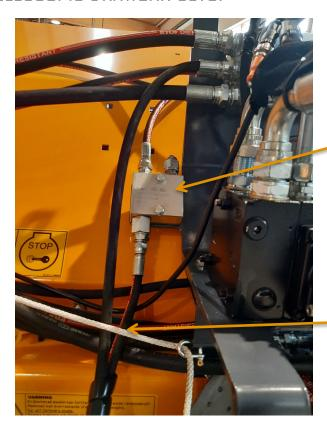
The pressure at which the telescopic drawbar extends is adjustable using this valve located on the right hand side of the main hydraulic block.
