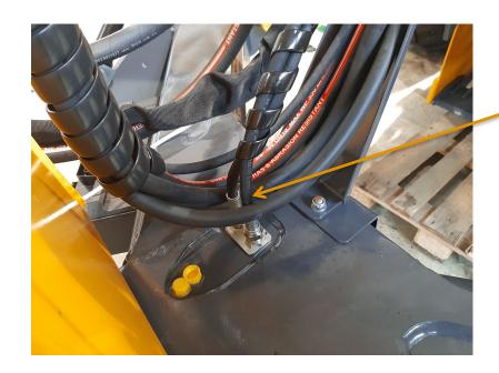
On the new drawbar the hoses for the telescopic cylinder go through the square pipe. One of the hoses connects to the valve adjusting the pressure when the telescope will extend. The other hose connects to a port marked T on the main block.
