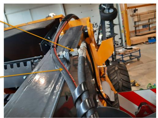
This hose is preconnected to the cylinders lifting the center elevator. The hose need to be attached securely at the rear for the bumper frame.
