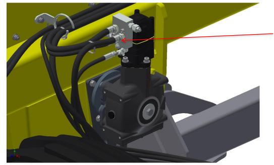
Connect the shorter hose (145743) from the rake motor to the outer port on the shockvalve for the main rotor motors.
