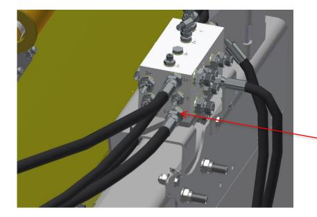
Connect the longer hose (145742) from the rake motors to the main block ports marked 1- for the right side rake and port 1- for the left side rake.
