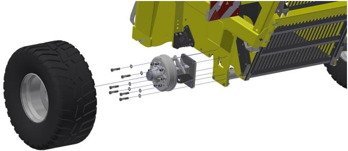
Attach the wheel axle using the 6xM24 bolts to 660 Nm. Attach the wheels using the eight wheel nuts, tighten to 450 Nm.
