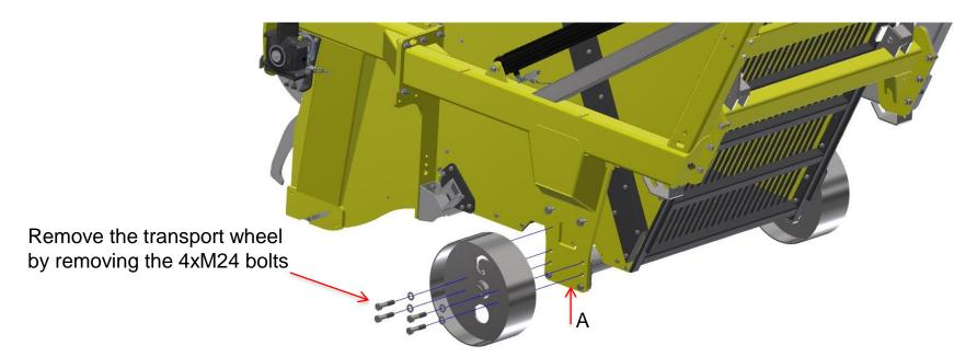
Take care when removing the transportation wheels and attaching the wheels. Make sure the machine is supported at point (A) before removing any parts. The distance between point A and the ground need to be **350-400 mm** for easy installation of the wheels.
