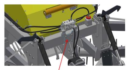
Attach the cover plate, part nr. 472665, with the supplied bolts and connect the bracket for the main hydraulic block.
